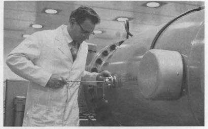
STEEL TANK, filled with carbon dioxide and nitrogen under high pressure, is checked by Herman Stein. The electric system enclosed in this tank permits a potential of more than two million volts.
